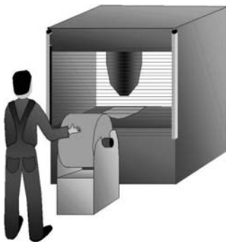
Figure 72 Typical application of "Floating Blanking" with "monitoring"
