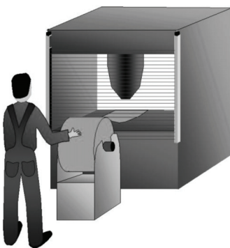
Figure 72: Typical application of "Floating Blanking" with "monitoring"
