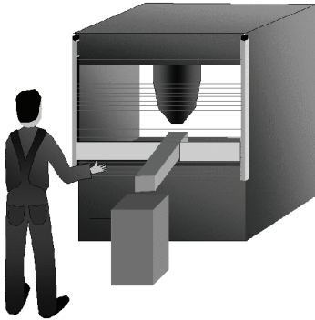
Figure 71: Typical example of "Fixed Blanking"
