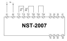
2-channel door monitoring with short circuit protection.
