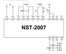
2-channel protection door monitoring with automatic activation and with opposite polarity between channels (Only NST-2007).
