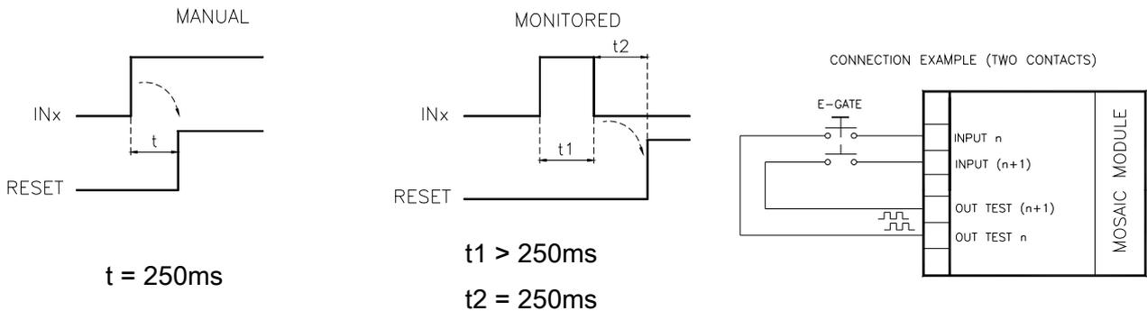
➔ **WARNING:** If the Manual Reset is active, a consecutive Input have to be used. Example : Input 1 and Input 2 are used for the functional block, then Input 3 have to be used for the Reset Input.
