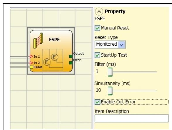
*Enable reset.* If selected this enables the request to reset each time the area protected by the safety light curtain is occupied. Otherwise, enabling of the output directly follows the input conditions.
