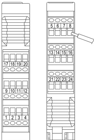
The DSC system units are provided with terminal blocks for the electrical connections. Each unit can have 8, 16 or 24 terminals.
