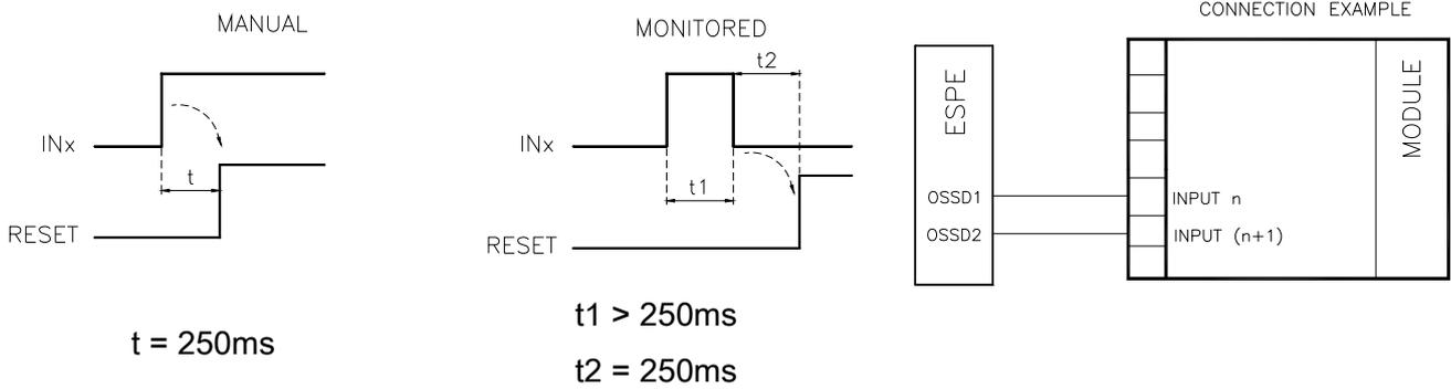
➔ **WARNING:** If the Manual Reset is active, a consecutive Input have to be used. Example : Input 1 and Input 2 are used for the fuctional block, then Input 3 have to be used for the Reset Input.
