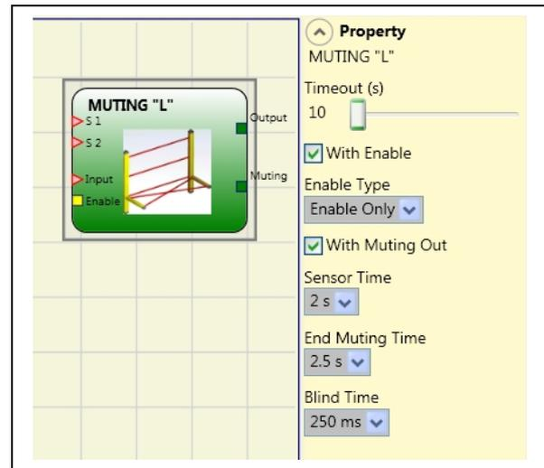
➔ Preliminary condition: The Muting cycle can only start if S1 and S2 are 0 (FALSE) and the inputs are 1 (TRUE) (barrier free).
