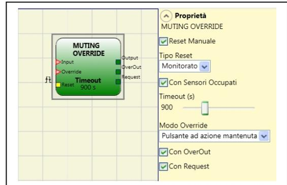
The operator must be connected after the Muting operator (Muting OUTPUT directly to the Override INPUT).
