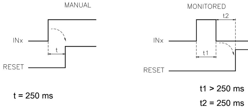
Important: for Manual reset always use the input immediately after those used by the function block. E.g.: if inputs 1 and 2 are used for the function block, use input 3 for Reset.
