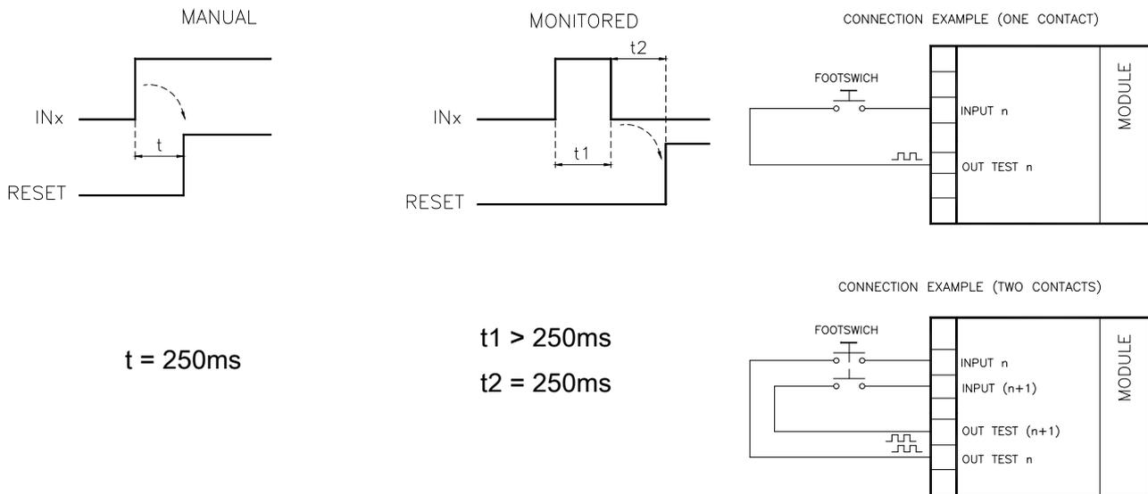
➔ **WARNING:** If the Manual Reset is active, a consecutive Input have to be used. Example : Input 1 and Input 2 are used for the fuctional block, then Input 3 have to be used for the Reset Input.
