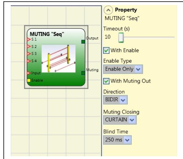
➔ Preliminary condition: The Muting cycle can only start if all the sensors are 0 (FALSE) and the inputs are 1 (TRUE) (barrier free).
