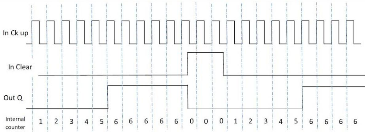
3) The counter generates a pulse duration equal to the system response time as soon as the set count is reached. If the CLEAR signal is activated, the internal count goes back to 0.
