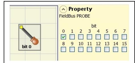
**WARNING:** the PROBE output is NOT a safety output
