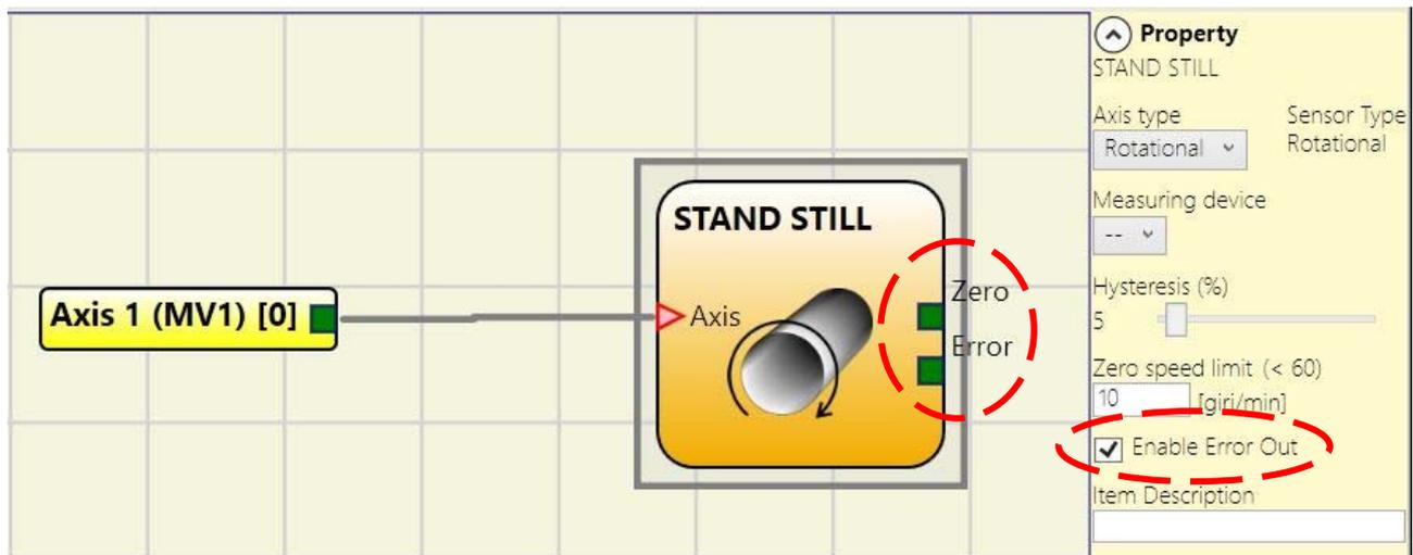
Figure 50 - Example of speed control functional block with Error Out enabled
