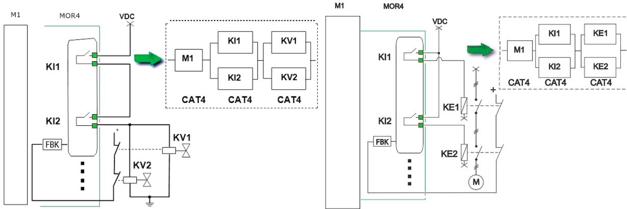
*External K delay (ms):* Select the Maximum delay the external contactors are allowed to introduce. This value can be used to check the maximum delay between switching of the internal relays and switching of the external contactors (during both activation and deactivation).
