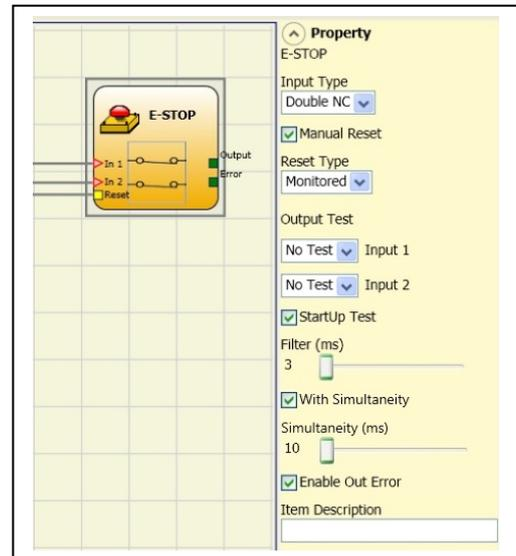
*Manual reset:* If selected this enables the request to reset each time the emergency stop is activated. Otherwise, enabling of the output directly follows the input conditions.
