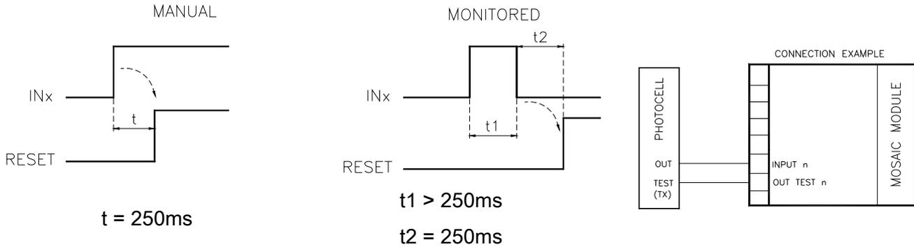
➔ **WARNING:** If the Manual Reset is active, a consecutive Input have to be used. Example : Input 1 is used for the fuctional block, then Input 2 have to be used for the Reset Input.
