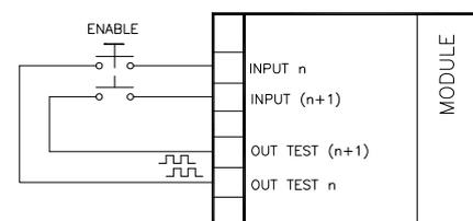
*Output test.* This is used to select which test output signals are to be sent to the component contacts. This additional control permits detection and management of any short-circuits between the lines. To enable this control, the test output signals must be configured (amongst those available).
