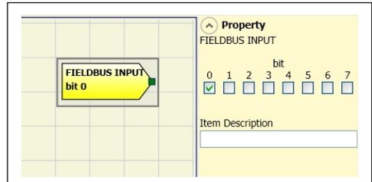
**WARNING:** the FIELDBUS INPUT is NOT a safety input.
