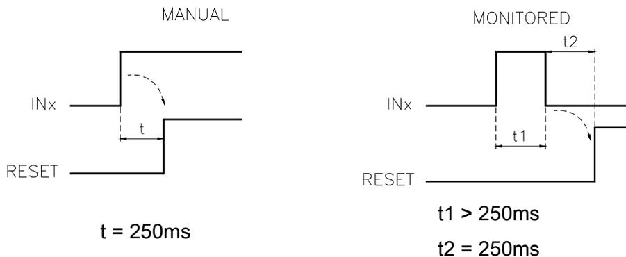
➔ **WARNING:** If the Manual Reset is active, a consecutive Input have to be used. Example : Input 1 is used for the fuctional block, then Input 2 have to be used for the Reset Input.
