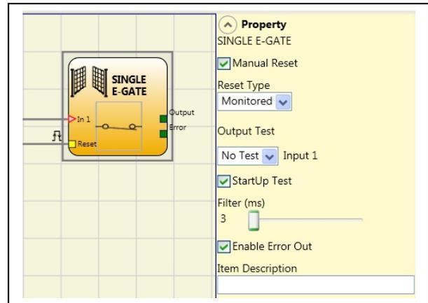
There are two types of reset: Manual and Monitored. When Manual is selected the system only verifies the signal's transition from 0 to 1. If Monitored is selected the double transition from 0 to 1 and then back to 0 is verified.
