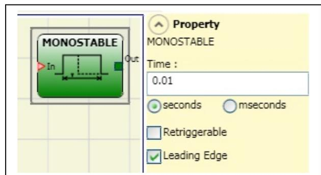
*Time:* The delay can be set to between 10 ms and 1093.3 s.
