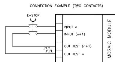
➔ **WARNING:** If the Manual Reset is active, a consecutive Input have to be used. Example : Input 1 and Input 2 are used for the functional block, then Input 3 have to be used for the Reset Input.
