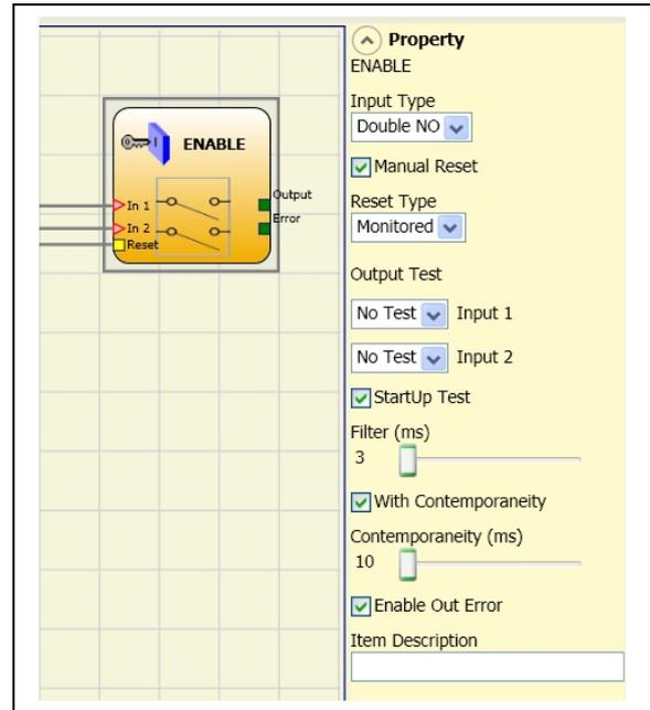
➔ **WARNING:** If the Manual Reset is active, a consecutive Input have to be used. Example : Input 1 and Input 2 are used for the functional block, then Input 3 have to be used for the Reset Input.
