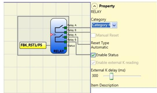
➔ In order to not affect the outcome of the calculation of the PL, the inputs (sensors or safety devices) must be of a category equal to or higher than the other devices in the chain.
