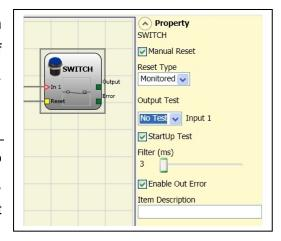
There are two types of reset: Manual and Monitored. When Manual is selected the system only verifies the signal's transition from 0 to 1.
