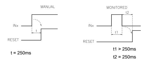
WARNING: if Reset is enabled, the input consecutive to those used by the functional block must be used. For example: if inputs 1 and 2 are used for the functional block, input 3 must be used for Reset.
