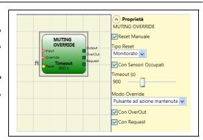
The operator must be connected after the Muting operator (Muting OUTPUT directly to the Override INPUT).
