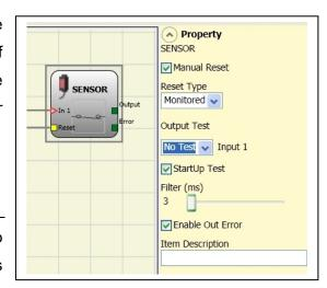
There are two types of reset: Manual and Monitored. When Manual is selected the system only verifies the signal's transition from 0 to 1. If Monitored is selected the double transition from 0 to 1 and then back to 0 is verified.
