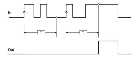
If not selected the logic is inverted, the output is set to 1 (TRUE) on the input signal's rising edge, the delay starts on the input signal's falling edge, at the end of the set time the output changes to 0 (FALSE) if the input is 0 (FALSE) otherwise it remains 1 TRUE.
