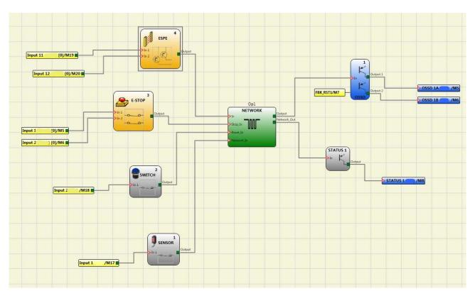
Figure 51 - Example of use of the NETWORK block
