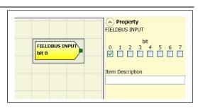
WARNING: the FIELDBUS INPUT is NOT a safety input.
