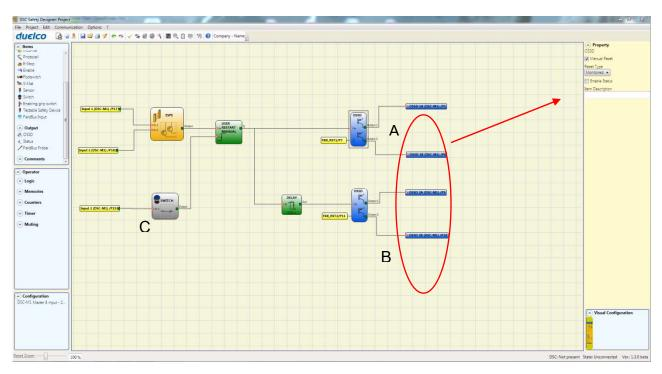
Figure 52 - Two outputs with one delayed (in MANUAL mode)
