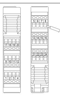
The DSC system units are provided with terminal blocks for the electrical connections. Each unit can have 8, 16 or 24 terminals.
