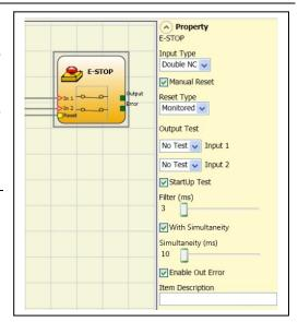
*Manual reset:* If selected this enables the request to reset each time the emergency stop is activated. Otherwise, enabling of the output directly follows the input conditions.
