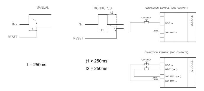
→ WARNING: If the Manual Reset is active, a consecutive Input have to be used. Example: Input 1 and Input 2 are used for the fuctional block, then Input 3 have to be used for the Reset Input.
