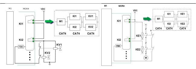
External K delay (ms): Select the Maximum delay the external contactors are allowed to introduce. This value can be used to check the maximum delay between switching of the internal relays and switching of the external contactors (during both activation and deactivation).
