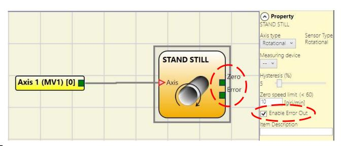
Figure 50 - Example of speed control functional block with Error Out enabled
