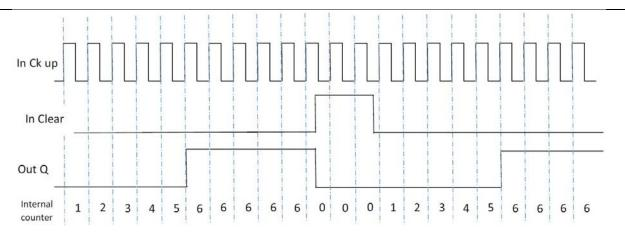
3) The counter generates a pulse duration equal to the system response time as soon as the set count is reached. If the CLEAR signal is activated, the internal count goes back to 0.
