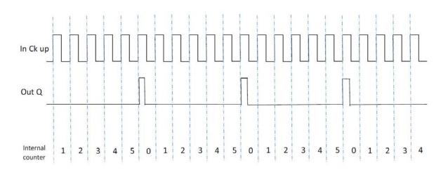
2) The counter leads to 1 (TRUE) the output Q as soon as it reaches the set count. The output Q goes to 0 (FALSE) when the signal CLEAR is activated.
