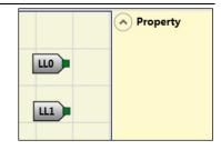
IMPORTANT: LL0 and LL1 cannot be used to disable the logical ports in the diagram.
