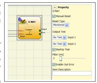
Monitored. When Manual is selected the system only verifies the signal's transition from 0 to 1. If Monitored is selected the double transition from 0 to 1 and then back to 0 is verified.
