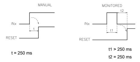
Important: for Manual reset always use the input immediately after those used by the function block. E.g.: if inputs 1 and 2 are used for the function block, use input 3 for Reset.
