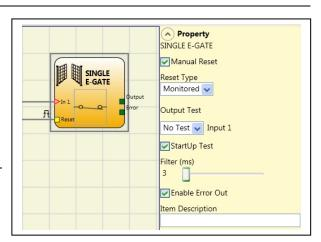
There are two types of reset: Manual and Monitored. When Manual is selected the system only verifies the signal's transition from 0 to 1. If Monitored is selected the double transition from 0 to 1 and then back to 0 is verified.
