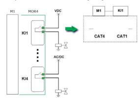
Category 2. Outputs with single Category 2 relay with OTE outputs. Each DSC-MOR4/S8 unit can have up to 4 of these outputs.
