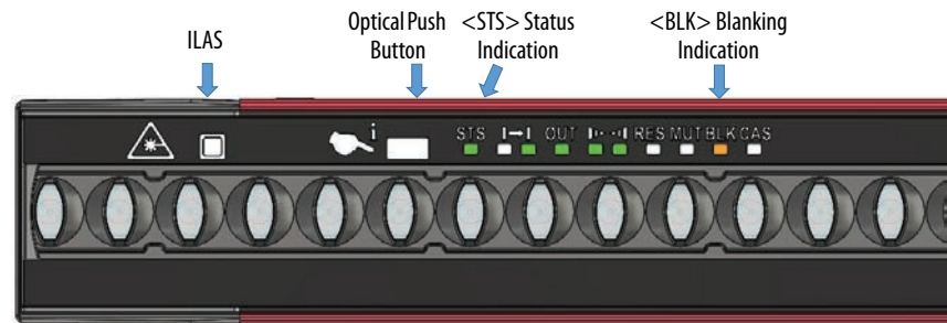
Figure 12 - Position of Optical Push Button, ILAS, and Status Indicators
