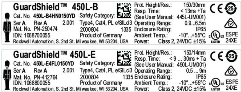
Figure 82 - 450L Transceiver Stick Label (Printed Since November 2018). Production date code: yyyy/mm/dd
