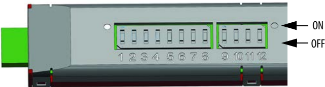
Figure 30 - DIP Switch Location at Receiver Plug-in
