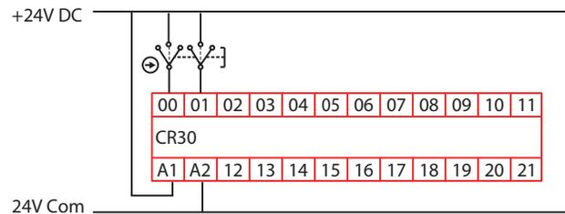
**Figure 43 - Example Schematic of a Dual Channel Enabling Switch Using Test Pulses A and B**
