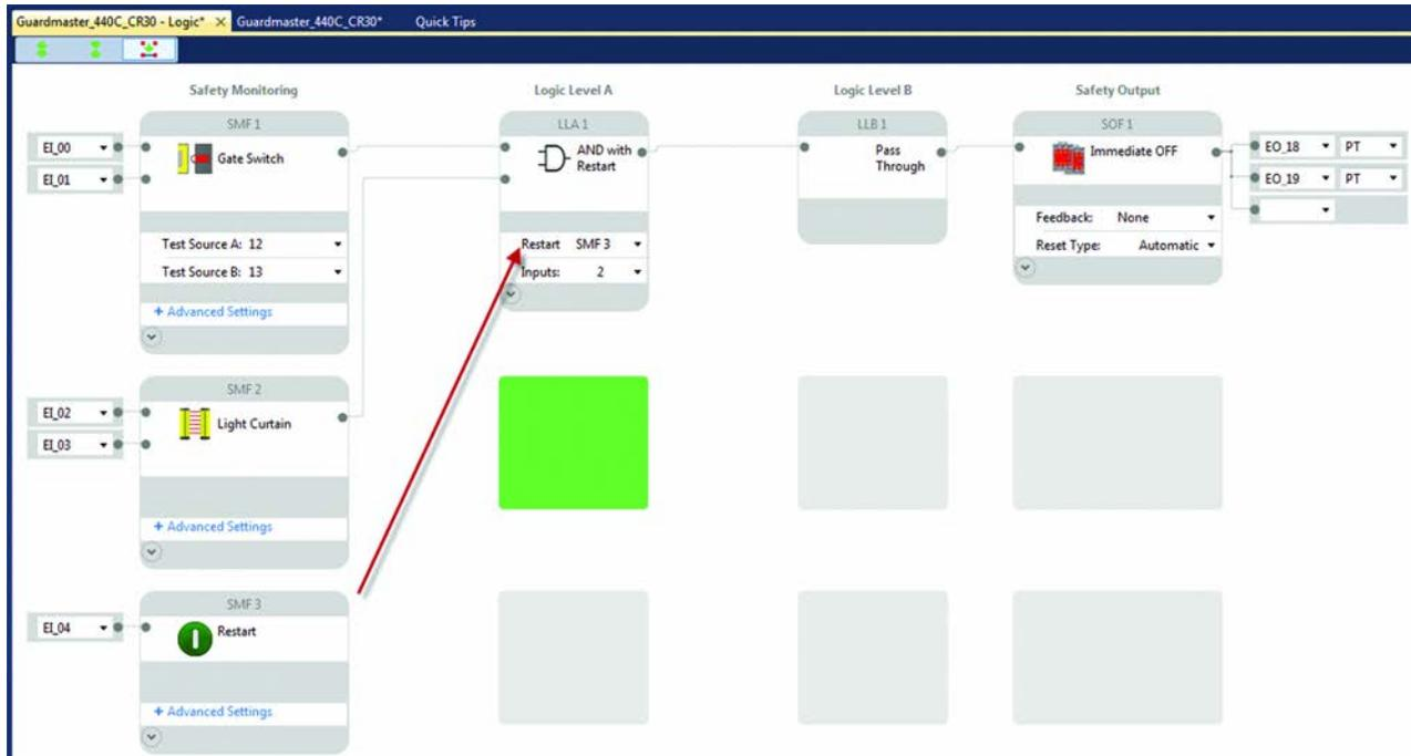
Figure 104 - Logic of the Restart Function with Two Input AND
