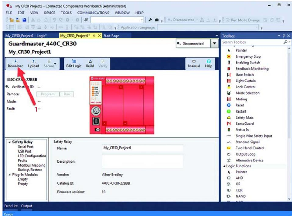
The configuration is built and the results appear in the Output pane. The Connection Browser window appears.
