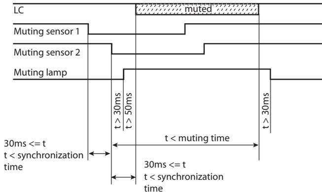
Table 7 shows the muting and synchronization times that are selectable in the Connected Components Workbench software. These times are selected independently. For example, you can select two-minute muting time, a 500-ms synchronization time between MS1 and MS2, and a 1000-ms synchronization time between MS2 and the light curtain.
