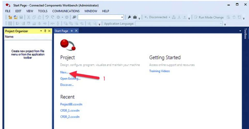
The Connected Components Workbench software maintains a list of projects to help prevent you from overwriting an existing project. The name of each new project increments by one (for example, Project90). This window allows you to select a name and a location for the file.
