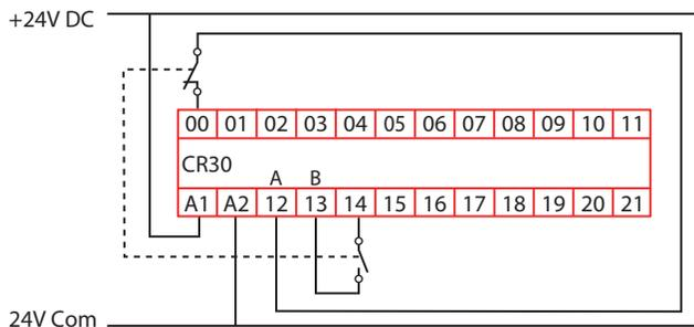
If a short circuit occurs on terminal 12 to 24V, the CR30 safety relay turns off its safety outputs within 35 ms. Remove the fault and cycle the contacts to clear the fault.
