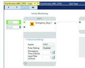
In [Figure 31](#), the Discrepancy Time is set to a nonzero value (enabled).
