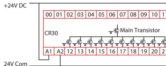
When the main transistor is tested, a 50- $\mu$ s test pulse appears simultaneously on all outputs. The main transistor is tested again 125 ms later.
