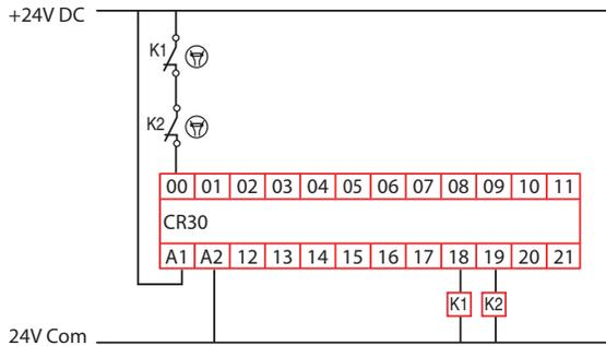
**Figure 46 – Example Feedback Schematic with Four Feedback Contacts Connected Individually to Four Input Terminals**
