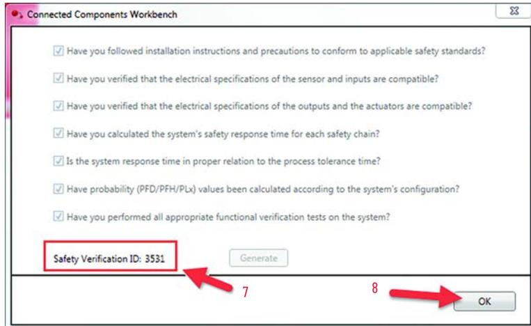
The ID is stored in the CR30 safety relay. During power-up, the CR30 safety relay uses this number during its self-testing to verify that its internal processors are functioning properly. When the configuration is uploaded from the CR30 safety relay, the Connected Component Workbench software shows the Verification ID.
