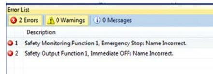
After clicking the Build button, the Error List shows the name errors. In the example in [Figure 37](#), SMF1 and SOF1 have naming errors.
