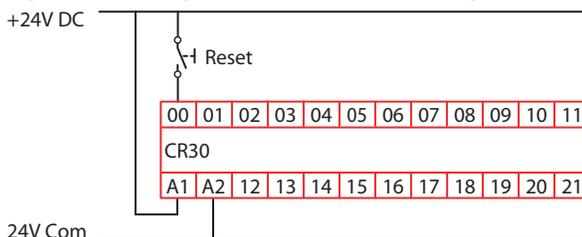
The reset block works with one or more output blocks. When an output block requires a manual reset, the Connected Components Workbench software shows all available reset inputs that can be used.
