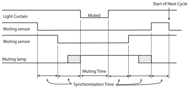
For proper operation, MS1 and MS2 must be activated/deactivated within the synchronization time, and the light curtain must be clear before the muting time expires.
