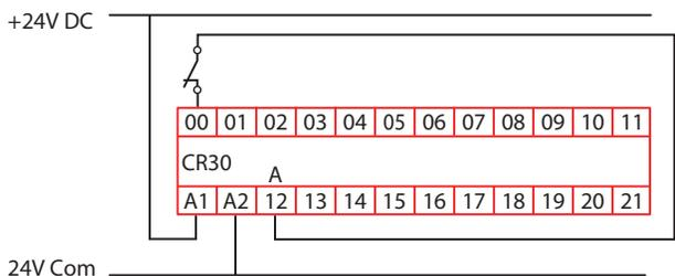
**Figure 90 - Example Schematic for Single Channel OSSD**
