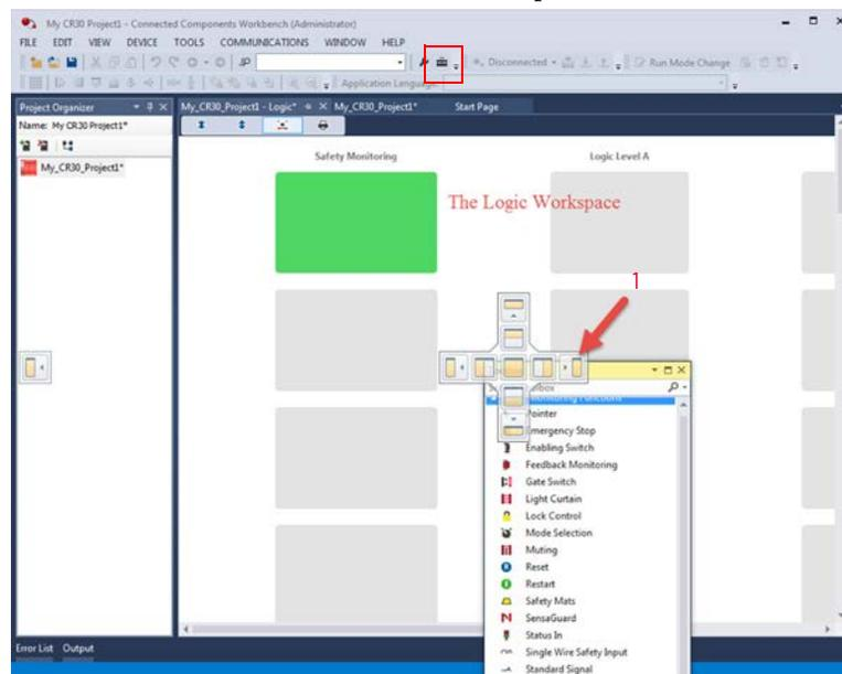
2. Click and drag the E-stop function block to the first block in the work space.
