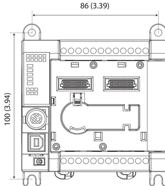
The preferred mounting method is to use four M4 (#8) screws per module. Hole spacing tolerance:  $\pm 0.4$  mm (0.016 in.).
