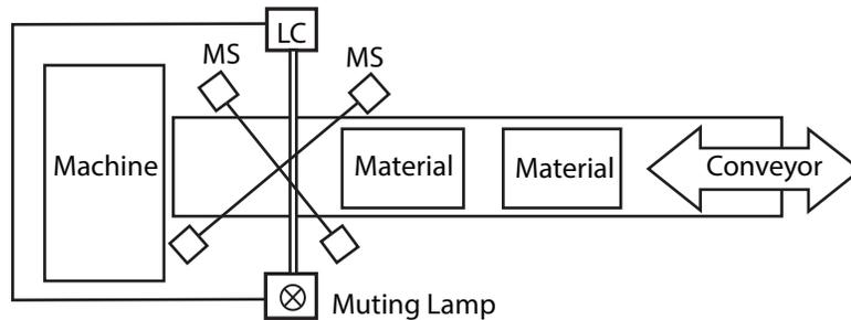
The material can break either MS1 first (or MS2 first), then the other sensor, and then the light curtain. As the material clears the light curtain, it must then clear MS2 (or MS1) first and then the other sensor. The muting lamp turns on shortly after the second sensor is blocked, and the light curtain is muted.
