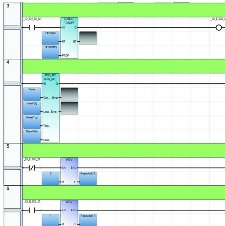
You must configure a second set of local variables. In this example, they are labeled `ResetCfg`, `ResetTrgt`, and `ResetAddr`.
