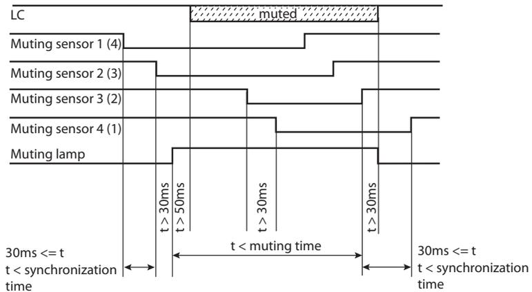
Table 8 shows the muting and synchronization times that are selectable in the Connected Components Workbench software. These times are linked. For example, if you select a 10-s muting time, then the synchronization time between MS1 and MS2 is 3 s. To use a synchronization time of 6 s, you must select a 60-s muting time.
