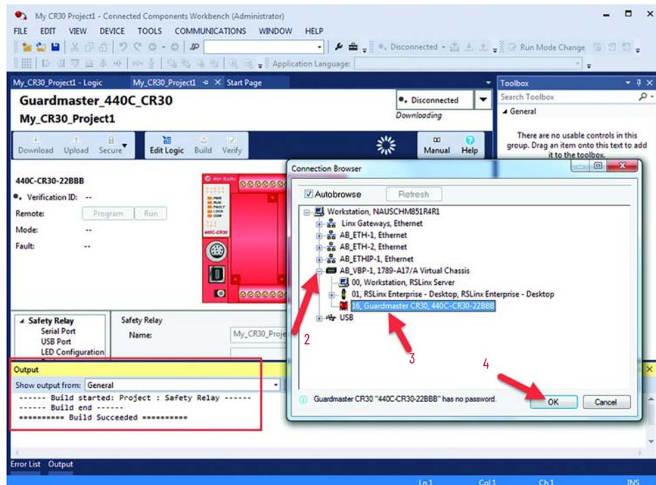
The configuration is downloaded to the CR30 safety relay. A dialog box with the Configuration CRC that was downloaded and the Configuration CRC that was uploaded as part of the verification process appears.
