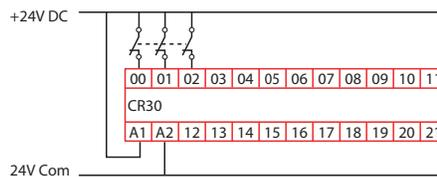
**Figure 98 - Example Schematic for Three N.C. with One Test Pulse Source**
