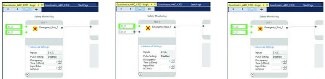
**Figure 34 - Discrepancy = Nonzero (Enabled) After the Initial Transition to Run Mode**
