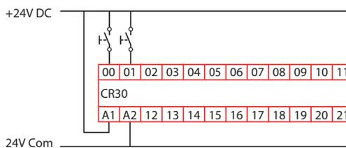
**Figure 83 - Wiring Connection for a Type IIIA Two-hand Control with the Test Pulses**
