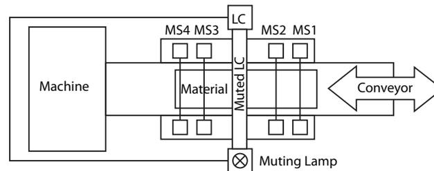
The material can travel in either direction; breaking MS1 first and MS4 last or breaking MS4 first and MS1 last. The muting lamp turns on and the light curtain is muted after the second sensor is blocked. The object must be large enough to break all four sensors.
