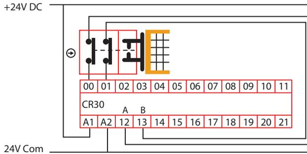
**Figure 50 - Example Schematic of a Dual Channel Safety Gate Switch Using OSSD Outputs**
