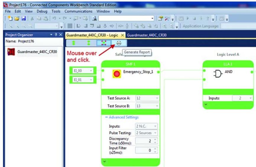
The report generator takes a snapshot of the logic editor as viewed by the operator. If the editor is actively monitoring the configuration, the report generator captures the colors reflected the block status. You can expand or collapse the blocks as desired to show or hide the advanced setting of each block.
