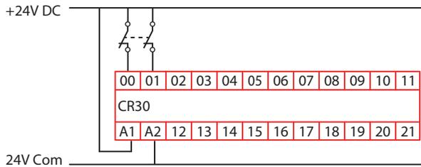
**Figure 92 - Example Schematic for 2 N.C. with Two Test Pulses Sources**
