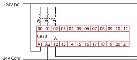
**Figure 99 - Example Schematic for Three N.C. with Three Test Pulse Sources**
