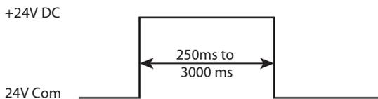
The reset block is a Safety Monitoring Function in the Connected Components Workbench software. For a valid Reset operation, according to the requirements specified in the approved safety concept, you must use the default Reset timing and leave the input filter setting “0”.
