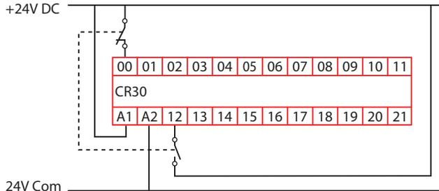
**Figure 95 - Example Schematic for N.C./N.O. with One Test Pulse**
