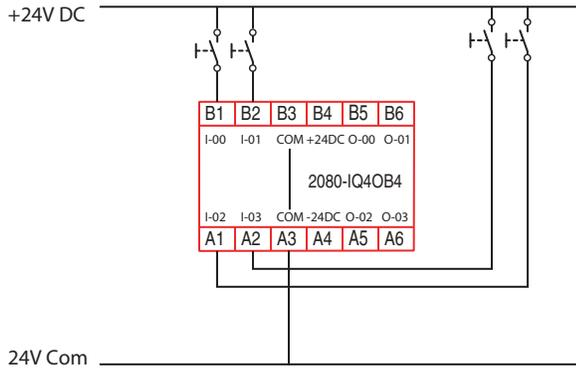
**Figure 122 - 2080-IQ4OB4 Schematic Showing Four Standard Output Signals**
