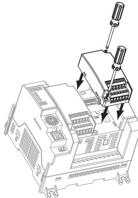
1. Position the plug-in module with the terminal block facing the front of the controller as shown.
