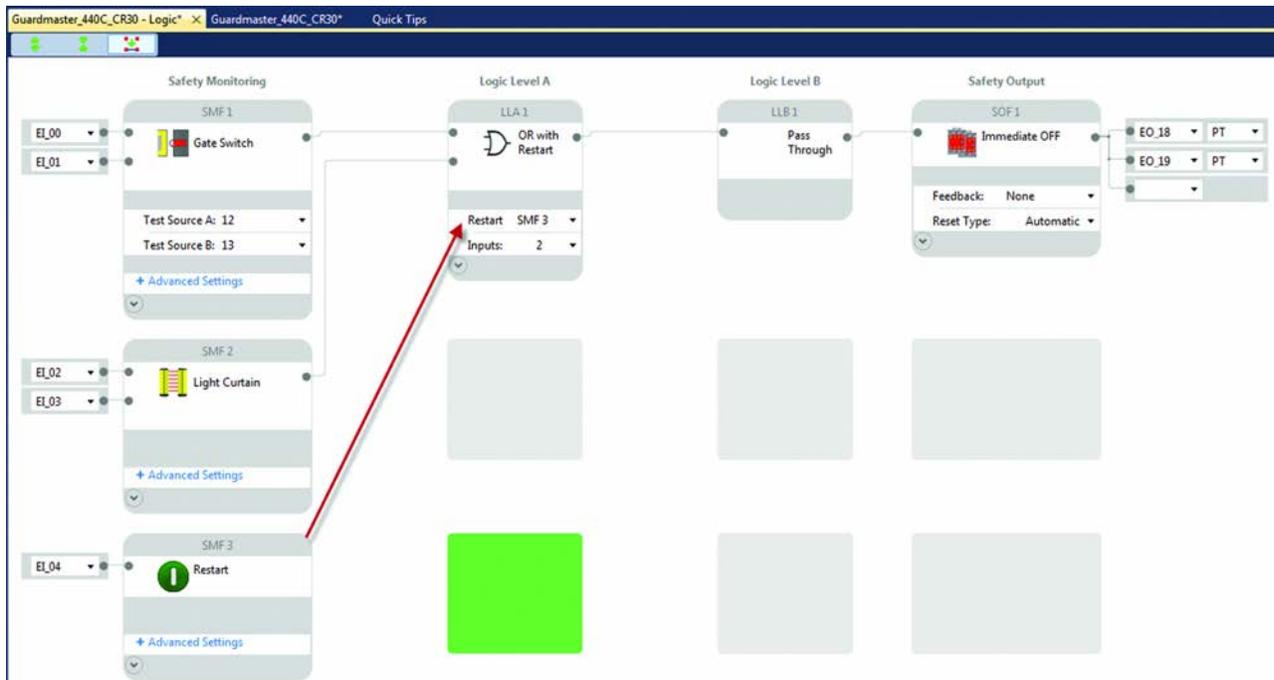
Figure 107 - Logic of the Restart Function with Two Input OR
