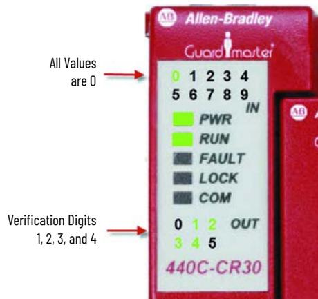
If the CR30 safety relay configuration has been verified, pressing the **Verification** button cycles the status indicators through each verification digit. In [Figure 15](#)...[Figure 18](#), the Verification ID is 7916.
