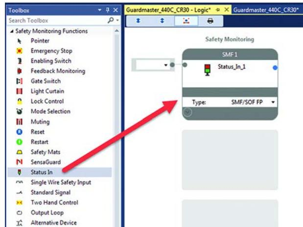
**Ready-for-reset** - In the Type field, select the **SOF RR** option. Then, assign an input to the desired Safety Output block.
