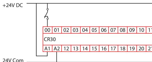
**Figure 89 - Example Schematic for Single-Channel N.C. with Test Pulse**
