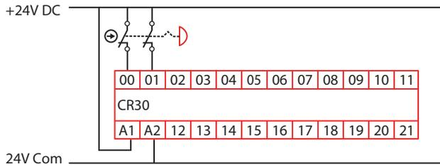
**Figure 40 - Example Schematic of a Dual Channel E-stop Using Test Pulses A and B**
