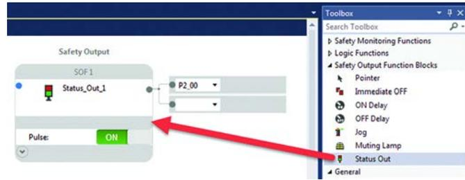
See [Figure 79 on page 73](#) and [Figure 80 on page 74](#) for examples of how the Status Out block works with the Status In block. [Figure 78 on page 73](#) shows how the Status Out block is used with other functions. In this example, the Status\_Out\_1 block pulses its output as soon as the E-stop button is pressed. When the E-stop button is released, the Status\_Out\_1 block turns OFF.
