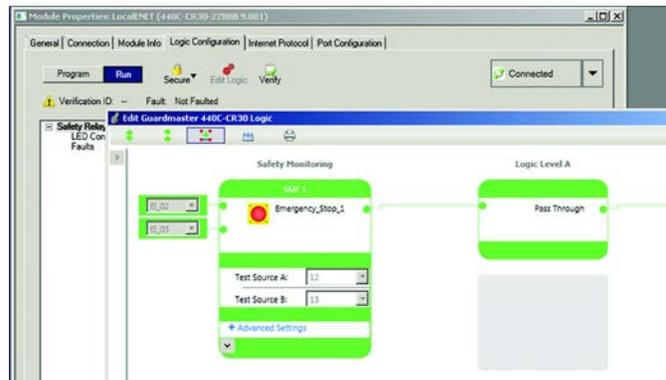
**IMPORTANT** After a download, the safety relay runs with the configuration for 24 hours without being verified. See [Verification on page 31](#) to learn more about how to verify the safety relay.
