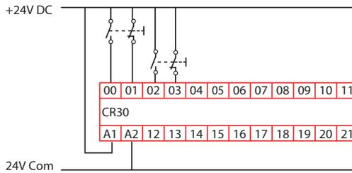
When test pulses are used, the CR30 safety relay detects a short from Channel 1 to Channel 2 after 3.7 seconds and turn the output OFF. To clear the fault, release both buttons.
