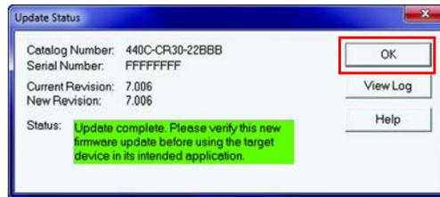
**IMPORTANT** If you see the following message, check the mode of the CR30 safety relay. ControlFlash cannot be performed when the CR30 safety relay is in run mode. The CR30 safety relay must be in program mode.
