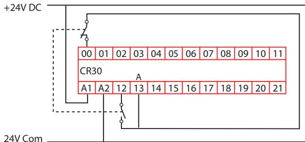
**Figure 96 - Example Schematic for N.C./N.O. with Two Test Pulses**
