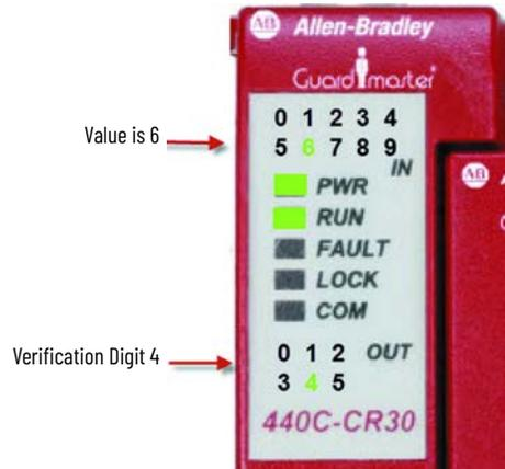
After 5 seconds, the status indicator revert to show the status of the inputs and outputs as configured in the Connected Components Workbench software.
