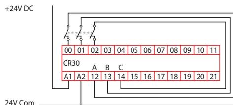
**Figure 100 - Example Schematic for Three OSSD**
