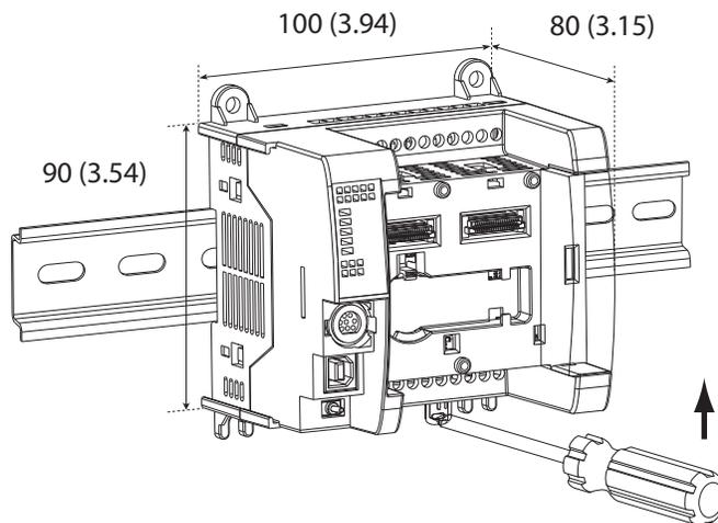
Maintain spacing from objects such as enclosure walls, wireways, and adjacent equipment. Allow 50.8 mm (2 in.) of space on all sides for adequate ventilation. If optional accessories/modules are attached to the relay, such as the power supply catalog number 2080-PS120-240VAC, make sure that there is 50.8 mm (2 in.) of space on all sides after attaching the optional parts.
