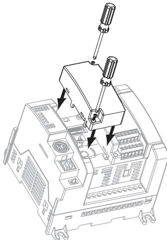
2. Snap the module into slot 1 of the module bay.
