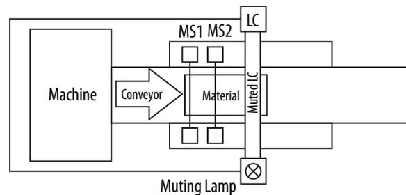
The material must first break MS1, then MS2 and then the light curtain. As the material progresses, the material must clear MS1 and then MS2. The muting lamp turns on and the light curtain is muted after MS2 is blocked. The conveyor can only move one direction.
