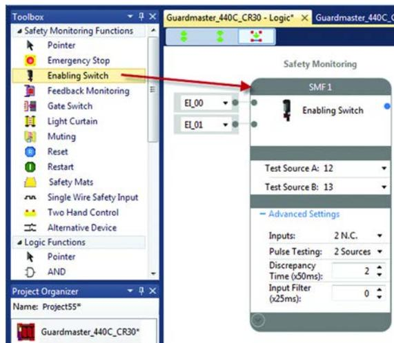
The available input selections for the Enabling Switch inputs are:
