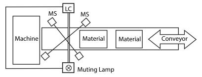
The material can break either MS1 first (or MS2 first), then the other sensor, and then the light curtain. As the material clears the light curtain, it must then clear MS2 (or MS1) first and then the other sensor. The muting lamp turns on shortly after the second sensor is blocked, and the light curtain is muted
