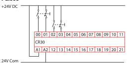
When test pulses are used, the CR30 safety relay detects a short from Channel 1 to Channel 2 after 3.7 seconds and turn the output OFF. To clear the fault, release both buttons.
