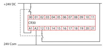
Figure 95 - Example Schematic for N.C./N.O. with One Test Pulse
