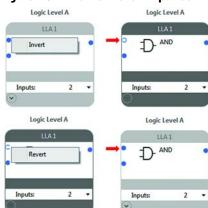
Figure 110 - Invert or Revert Input Connection Points
