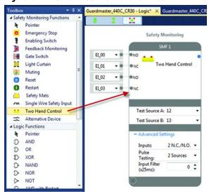
The two-hand controls can be connected to the following terminals.
