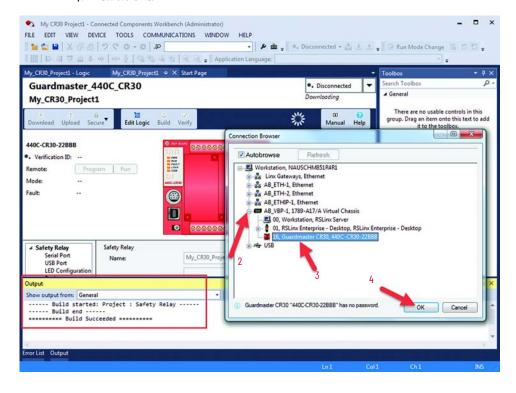
The configuration is downloaded to the CR30 safety relay. A dialog box with the Configuration CRC that was downloaded and the Configuration CRC that was uploaded as part of the verification process appears.
