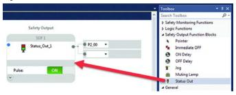
See <u>Figure 79 on page 73</u> and <u>Figure 80 on page 74</u> for examples of how the Status Out block works with the Status In block. <u>Figure 78 on page 73</u> shows how the Status Out block is used with other functions. In this example, the Status\_Out\_1 block pulses its output as soon as the E-stop button is pressed. When the E-stop button is released, the Status\_Out\_1 block turns OFF.
