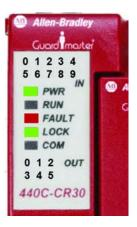
The status indicators are as follows: PWR - steady green RUN - off (not executing) FAULT - steady red LOCK - steady green
