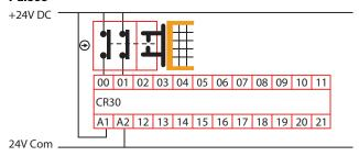
Figure 49 - Example Schematic of a Dual Channel Safety Gate Switch Using Test Pulses A and B
