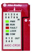
The status indicators are as follows: PWR - steady green RUN - off (not executing) FAULT - steady red LOCK - steady green COM - off
