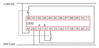
If a short circuit occurs on terminal 12 to 24V, the CR30 safety relay turns off its safety outputs within 35 ms. Remove the fault and cycle the contacts to clear the fault.
