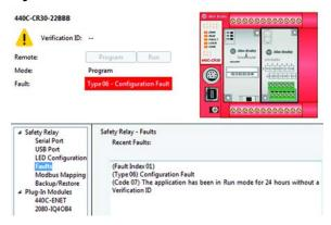
If the safety system is verified, the CR30 safety relay assigns a four-digit number and allows the relay to operate in Run mode beyond the 24-hour limit. After verification, the Run status indicator remains steady green.
