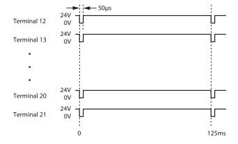
Then a sequence occurs in which each output is individually tested twice. The test pulse is 50  $\mu$ s wide. The test pulses occur every 250 ms and switch to the next output configured with testing.
