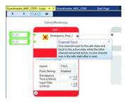
Both channels start from a HI state. One input goes LO and stays LO after the discrepancy time. This action generates a Discrepancy Fault.
