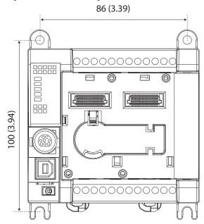
The preferred mounting method is to use four M4 (#8) screws per module. Hole spacing tolerance: ±0.4 mm (0.016 in.).
