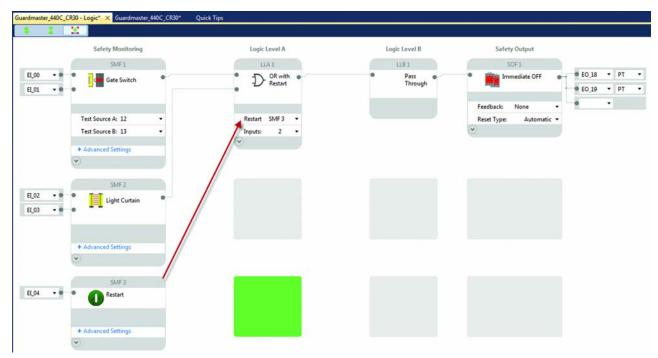
Figure 107 - Logic of the Restart Function with Two Input OR
