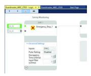
In <u>Figure 31</u>, the Discrepancy Time is set to a nonzero value (enabled).
