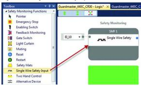
Only terminals 10 and 11 of the CR30 safety relay can be configured to receive the SWS signal.
