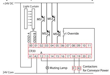
For simplicity, the power and ground connections of the light curtain and muting sensors are not shown. The light curtain and muting sensors must have the same reference (24V Com) as the CR30 safety relay for proper operation.
