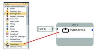
Any single SOF can be the input on multiple output-loop safety-monitoring functions.
