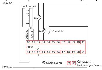
For simplicity, the power and ground connections of the light curtain and muting sensors are not shown. The light curtain and muting sensors must have the same reference (24V Com) as the CR30 safety relay for proper operation.
