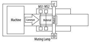
The material must first break MS1, then MS2 and then the light curtain. As the material progresses, the material must clear MS1 and then MS2. The muting lamp turns on and the light curtain is muted after MS2 is blocked. The conveyor can only move one direction.
