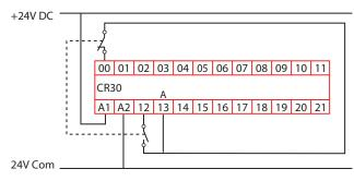
Figure 96 - Example Schematic for N.C./N.O. with Two Test Pulses
