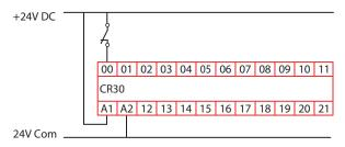
Figure 89 - Example Schematic for Single-Channel N.C. with Test Pulse
