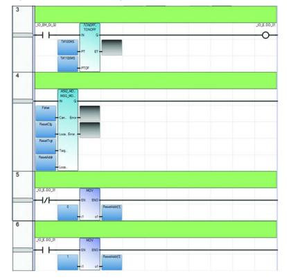
Figure 137 - Reset Ladder Diagram
