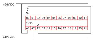
Figure 90 - Example Schematic for Single Channel OSSD
