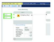
Both channels start from a HI state. One input goes LO and stays LO. Notice that one input is gray and the second input is green. The SMFI output is OFF, and no fault is present.
