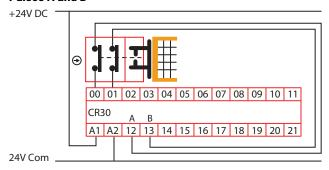
Figure 50 - Example Schematic of a Dual Channel Safety Gate Switch Using OSSD Outputs
