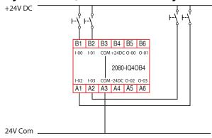
Figure 122 - 2080-IQ40B4 Schematic Showing Four Standard Output Signals
