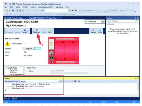
7. The function blocks are colored to indicate their status. All blocks are green, which indicates the dual E-stop circuits are closed and the output terminals are ON.
