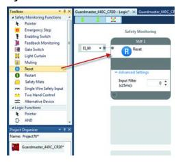
To help prevent inadvertent actuation of the reset block, the reset requires a leading and trailing edge within a specific time frame. The pulse width must be between 250...3000 ms. If the pulse width is too short or too long, the reset function is not executed.
