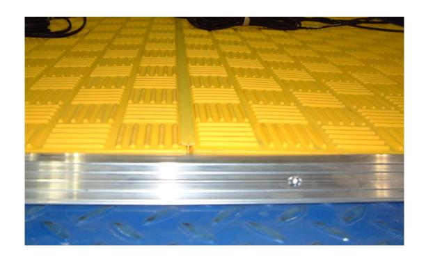
The 45 degree mitre at the end of the Active Uniting Strip increases the flexibility at the join allowing the mat to be easily pressed down and slid underneath the Perimeter Trim which will sit with its support legs flush to the floor. The 45 degree mitre ensures that the mat is not clamped too tightly at this point.
