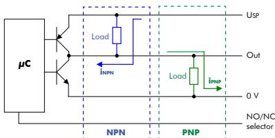
Rx cable connection of the load:
