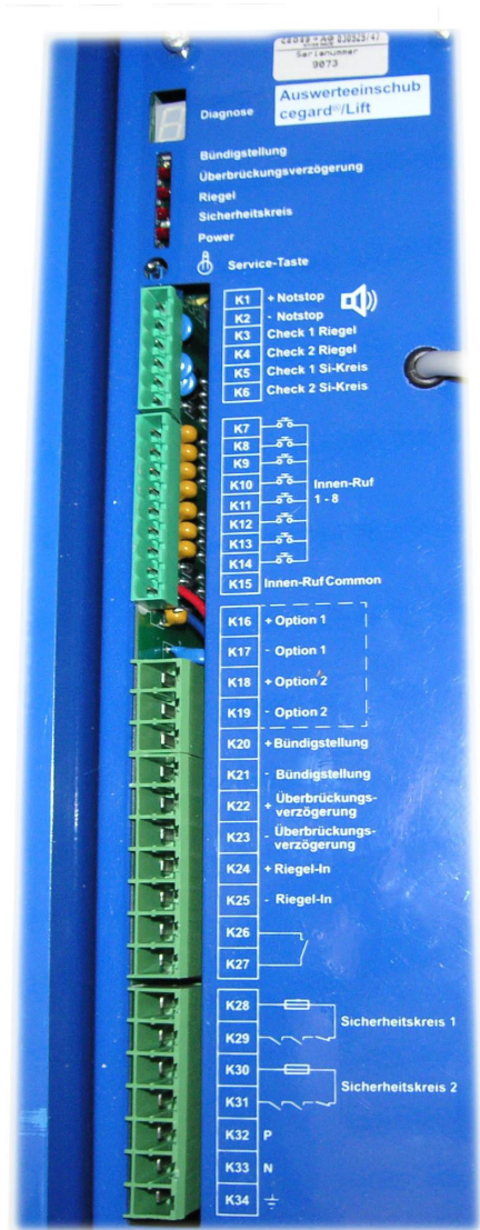
Figure 10: Connection terminals plug-in system controller
